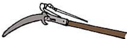
Figure 2. Combination pole saw pruner
